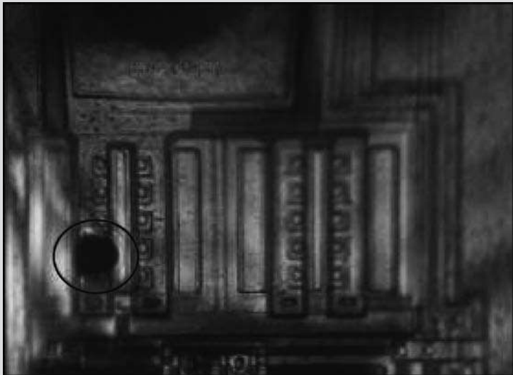
Figure 13.13 Liquid Crystal Thermography uses temperature sensitive chemicals and polarized cameras to detect hot spots on the die surface.
