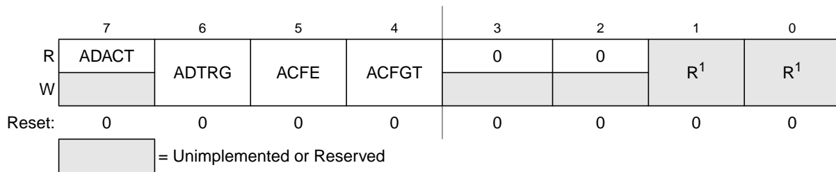
Figure 9-4. Status and Control Register 2 (ADCSC2)
